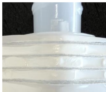
sealing at 0,5 sec., 200°C VISIBLE DAMAGE
